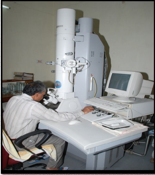
OBSERVATION OF STAINED GRIDS UNDER TRANSMISSION ELECTRON MICROSCOPE (TEM)- HITACHI-H-7500
