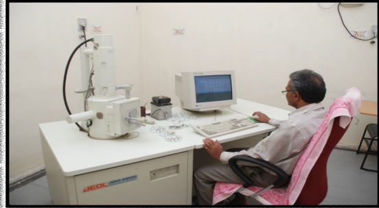
OBSERVATION UNDER (SEM )- SCANNING ELECTRON MICROSCOPE JEOL - JSM - 5600
